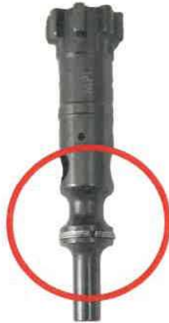
Incorrectly Staggered Gas Rings
